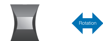
▲ Bi-directional x-tooth, for dispersers that change direction of rotation
