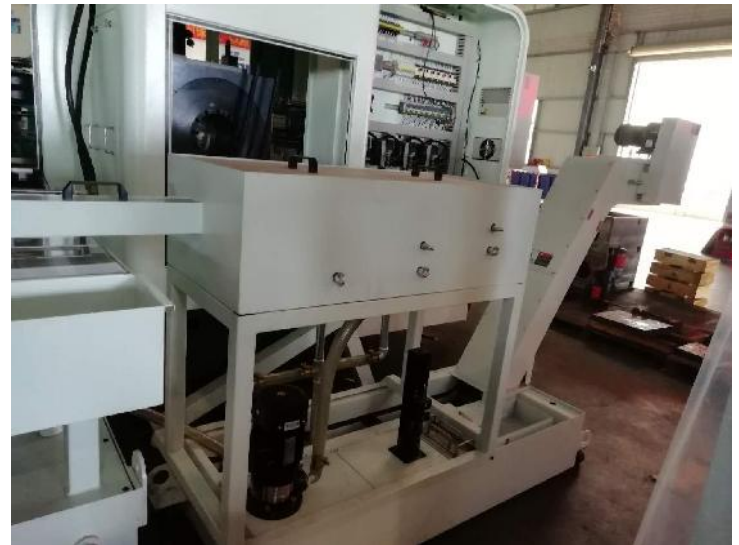
Automatic Scrapes Removal System
